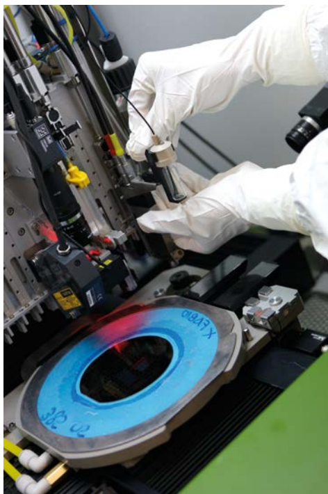
Micro dispensing on wafer.
